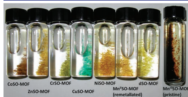
Figure 1. Digital photographs of vials containing solvated crystals of (right to left, as labeled) the \text{Mn}^{III}\text{SO-MOF} parent, dSO-MOF, and MSO-MOFs after remetalation. There is a clear difference in color between the parent \text{Mn}^{III}\text{SO-MOF} and the remetalated \text{Mn}^{II}\text{SO-MOF} (third from the right).
